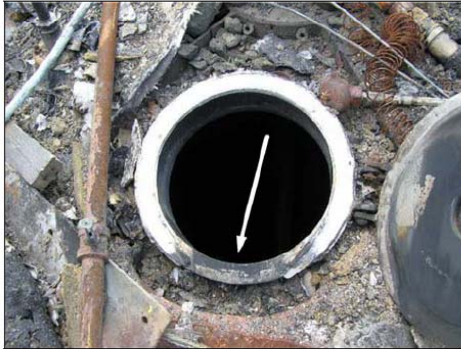
Figure 6. Damaged manway gasket, showing vapor release path
